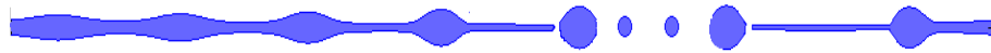
Figure 2.2: A schematic depicting the breakup of a liquid jet under the Rayleigh regime with subsequent main and satellite drop formation. Notice how breakup occurs many jet diameters away from the orifice (far left of picture) and droplet sizes are comparable to the jet radius.
