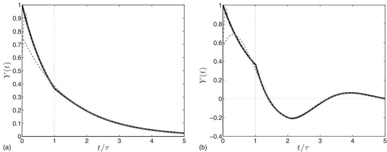
FIG. 1. The fundamental solution,  $Y(t)$ , plotted as a function of  $t/\tau$  (solid black line). Also plotted are  $Y_1(t)$  (dashed gray line) and  $Y_5(t)$  (dashed-dotted gray line) [see Eq. (15b)]. In both parameter sets  $\text{Re } \lambda_1 \approx -0.68$ .
