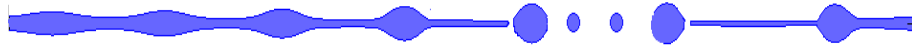
Figure 2.2: A schematic depicting the breakup of a liquid jet under the Rayleigh regime with subsequent main and satellite drop formation. Notice how breakup occurs many jet diameters away from the orifice (far left of picture) and droplet sizes are comparable to the jet radius.
