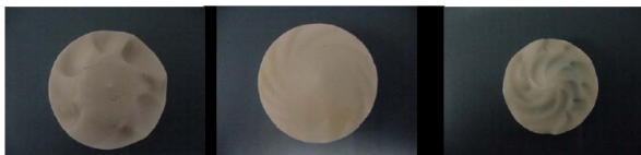
Figure 4: Dimpled structures observed on carbonate rotating disk heads caused by mass transfer of acidic solutions during drilling process. Picture courtesy of Frank Chang (Schlumberger).
