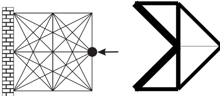
Figure 3: Three-by-three truss with nonstructural mass (Ex. 4.2): initial layout and optimal topology
