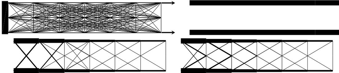
Figure 10: A medium size multiple-load example (Ex. 4.7): initial layout (top-left); optimal topology without (top-right) and with (bottom-left) vibration constraints; single-load optimal result with vibration constraints (bottom-right)
