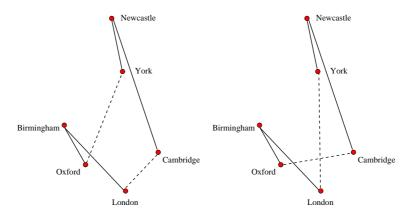
For a general TSP if the current tour contains edges AB and CD, then the 2-interchange operations means replacing these edges with AC and BD.
