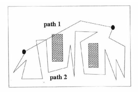
Which path is better for the robot? Altough path 2 is feasible and path 1 is infeasible, path 1 is much shorter and smoother than path 2. Moreover, path 1 can be easily repaired (a small deviation of path 1 around the corner of the crossed obstacle is enough to make it feasible). Moreover, the repaired version of path 1 is much better than path 2.
