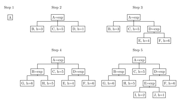
At Step 2 we expand node A, put it in the closed list and put its successors B, C, D in the open list. The closed list becomes CLOSED=(A) and the open list OPEN=(B,C,D). We have to choose the node in the open list with the lowest h value, that is, D.
