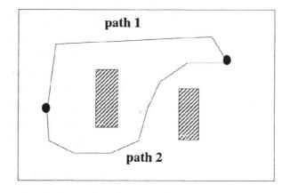
When evaluating a path we need to consider criteria such as the total distance, clearance from obstacles and smoothness. Based on these criteria, the two paths in the previous figure are contradictory. Indeed, although path 1 is shorter and seems more clear from obstacles (it goes around one obstacle only, while path 2 goes around both obstacle), path 2 is smoother.
