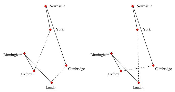
Recall the more precise definition of the 2-interchange operation. If AB and CD are two non-adjacent edges in a tour, by 2-interchange we mean replacing AB and CD with AC and BD and leaving all other edges unchanged.
