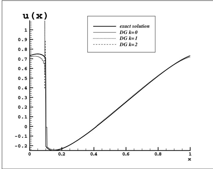
FIG. 2. Exact and numerical solution to the Burgers equation. Smooth approximation to the solution generates local oscillations at the shock for the DG solution with polynomial degree  $K > 0$ . The solution overshoots can be eliminated by means of local limiters.
