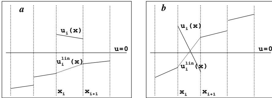
FIG. 4. Examples of nonphysical flux extrema in the problem (18), (9). (a) The subsonic solution overshoot produces a sonic point and a shock at the cell interfaces. (b) The sonic solution overshoot produces a shock at the interior point of the cell and another sonic point at the cell interface.
