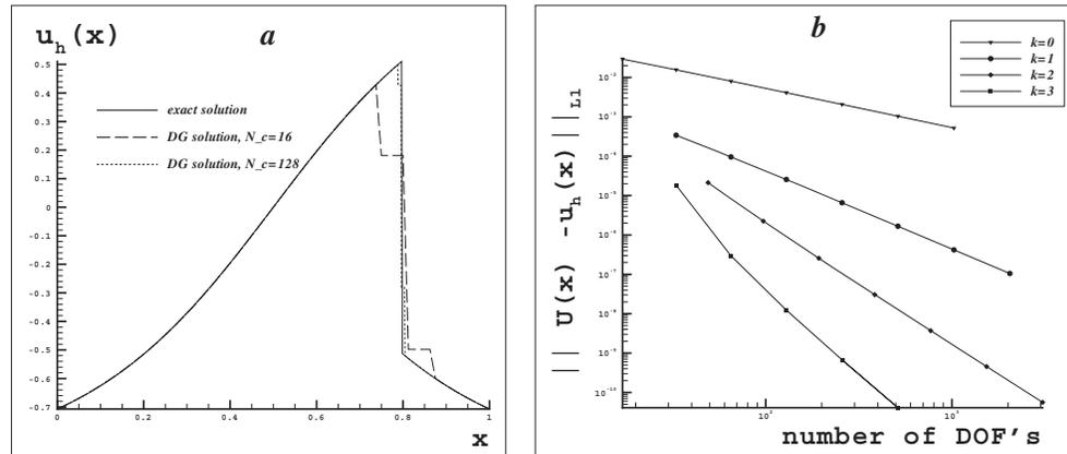
FIG. 5. Numerical solution to the problem (18), (9). (a) An example of the DG solution (polynomial degree  $K = 3$ ) on a coarse and a fine grid.  $N_c$  is the number of grid cells. (b) Convergence history for the DG solution with polynomial degree  $K \geq 0$ .
